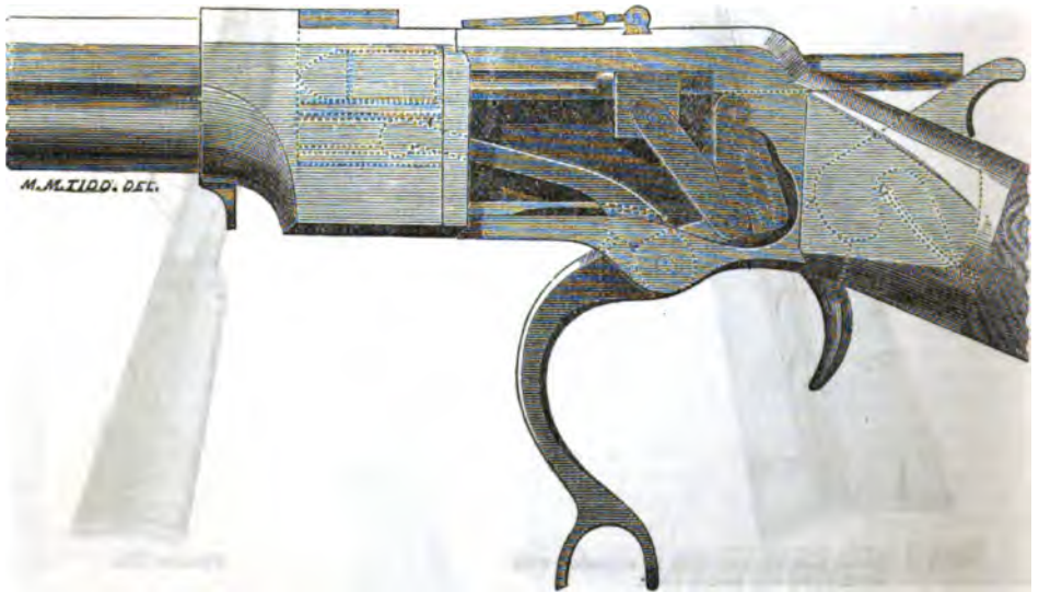
Sectional view of working parts, showing the operation of removing the empty cartridge and cocking the hammer.
